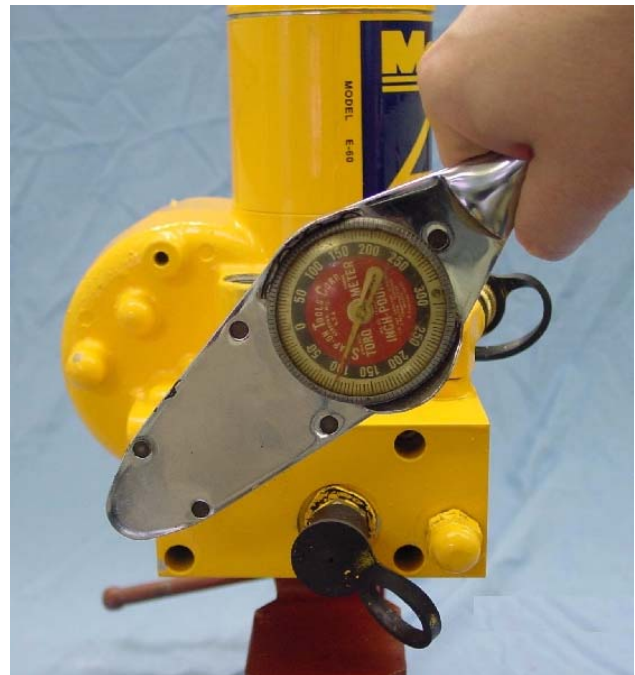
FIGURE 3-71 Install P.A. Block Assembly using 5/16-18 x 1-1/2" soc. head screws. Torque to 96-120 in. lbs.
