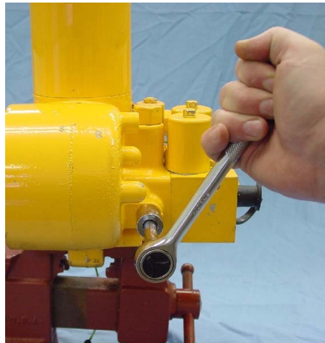
FIGURE 3-17 Remove Pressure Port Filter Cap Nut.
