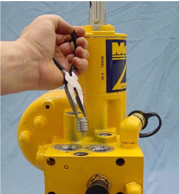
FIGURE 3-32 Pilot Check Piston being removed. Handle Piston with care. If Piston is scratched or damaged, it must be replaced.
