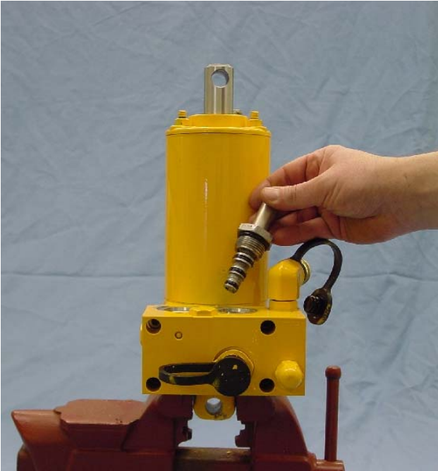
FIGURE 3-30 Remove "C" Cartridge from Sump Base.
