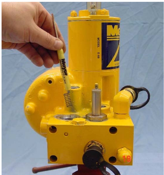
FIGURE 3-28 Remove "B" Check Valve Spring from Valve Body.
