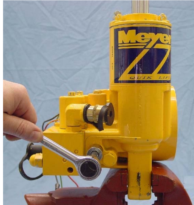
FIGURE 3-15 Remove the Lower Adjusting Screw Cap Nut using a 11/16" hex socket.
