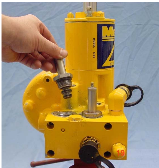
FIGURE 3-26 Remove "B" Cartridge from Sump Base.
