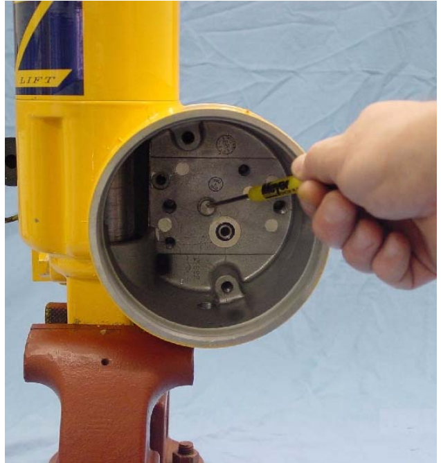
FIGURE 3-11 Remove Pump Mounting Plate Locator Pin.
