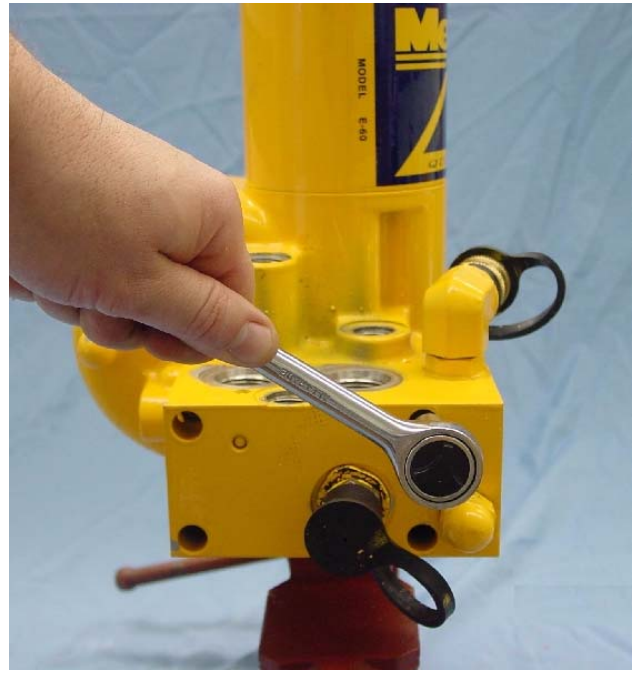
FIGURE 3-33 The Valve Body can be removed from Sump Base using a 1/4" Allen wrench.
