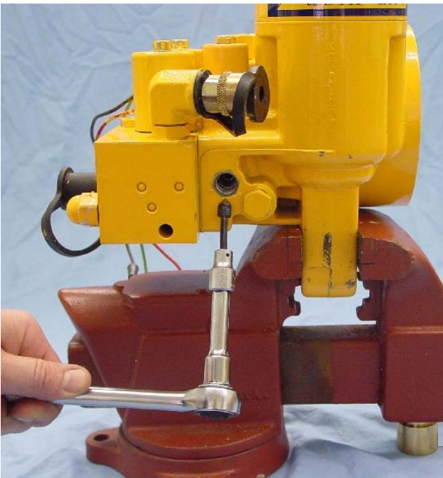
FIGURE 3-16 Directly beneath the Cap Nut is the location of the Lower Adjustment Screw. Remove the Lower Adjustment Screw from the Sump Base using a 3/16" Allen wrench.
