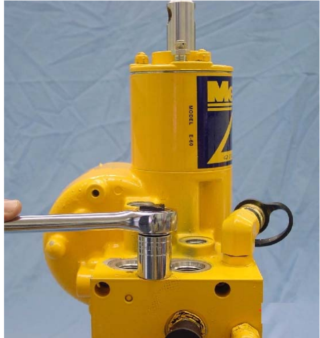
FIGURE 3-31 Use a 13/16" hex socket to remove Pilot Valve Plug.
