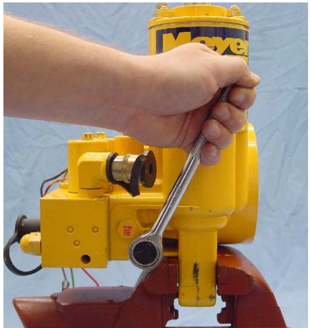
FIGURE 3-13 There are two filters located within the E-60 and E-60H units. Remove Lower Filter Cap Nut using a 11/16" hex socket.
