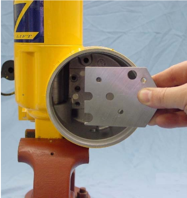
FIGURE 3-10 Remove Pump Mounting Plate.
