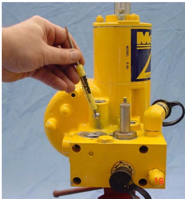
FIGURE 3-27 A magnetic probe is useful for removal of small parts. Remove the 7/16" Ball located directly beneath the "B" Cartridge
