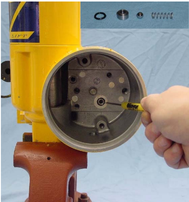
FIGURE 3-12 Remove Pump Check Valve.
